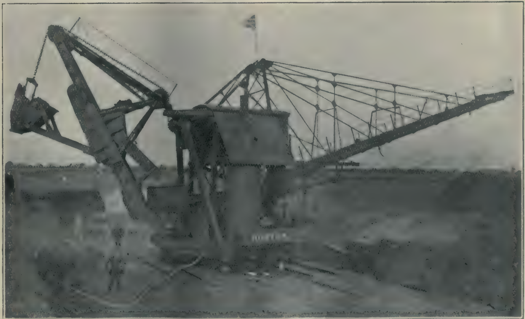
FIG. 4—Another type of machine for dealing with the cover, consisting of a digger and transporter combined.
